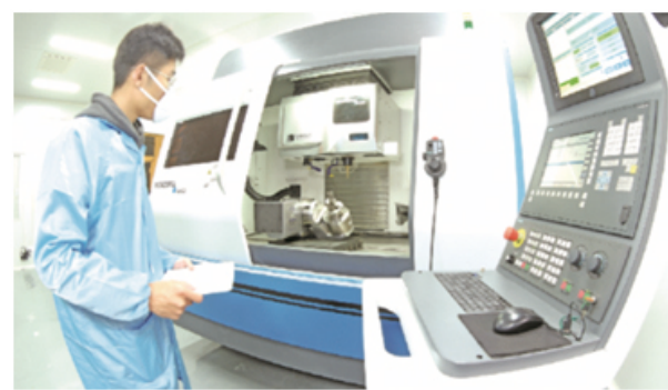
飞秒激光切割航天推进器过流片。商维中摄
